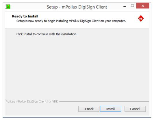
5. To start the installation, click **Install**. The installation program starts installing the software and shows the release notes after the installation is completed. After the installation, these notes can be found in the DigiSign Client directory as ReleaseNotes.txt.
